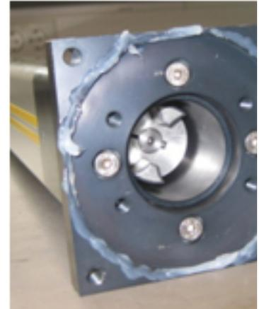
Figure 28: Flange prepared for IP65
